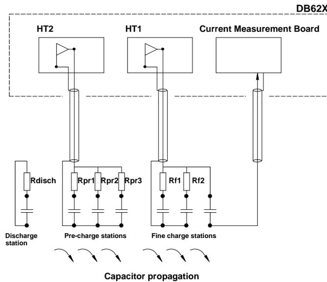
Fig. 1: Example of IR testing set-up.
